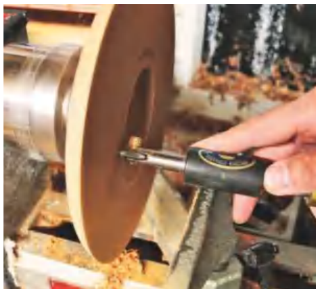
▲ Working the face on this softer sapele gives fast results
